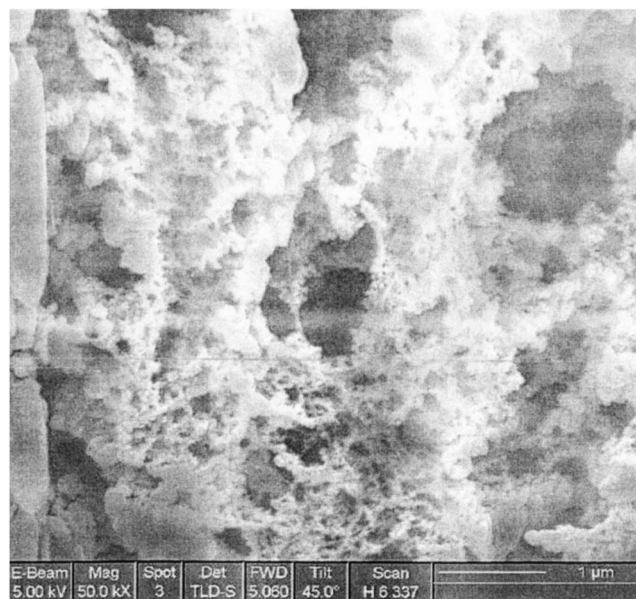
FIG. 2. Cross-sectional SEM of cottonlike \text{SiO}_x thin film, on cutting by a focused Ga-ion beam.
