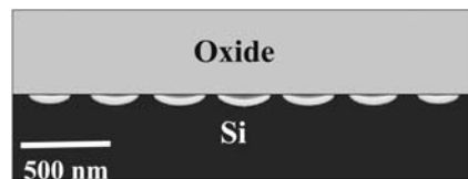
FIGURE 4 Cross-sectional (along y -axis) image, showing the solid/liquid coexisting of the laser irradiated area, was obtained by numerical simulation
