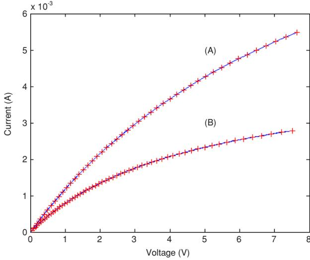
**Figure 1.** Current–voltage ( $I$ – $V$ ) plots of the analytical approximation (line) and numerical solution (crosses) of equation (3) for a typical laser-diffused resistor: (A)  $N_D = 5 \times 10^{18} \text{ cm}^{-3}$ ,  $L = 0.6 \mu\text{m}$  and (B)  $N_D = 1 \times 10^{18} \text{ cm}^{-3}$ ,  $L = 1.7 \mu\text{m}$ . (This figure is in colour only in the electronic version)
