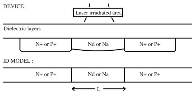
**Figure 2.** Schematization of the 1D model applied to the geometry of a laser-diffused resistor.
