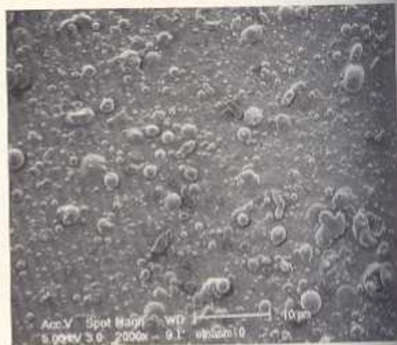
Fig. 2. Micrograph of a NASICON thin film deposited at 1.5 \text{J}/\text{cm}^2 on a Raipore membrane.
